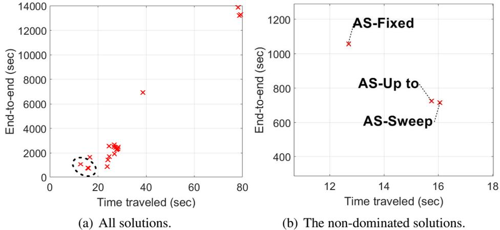
Figure 7: The objective space of the case where tasks arrive with  $\alpha$ . The polices form a Pareto frontier as marked in (a). The three polices correspond to the fixed- $x$ , up-to- $x$ , and the sweeping policy with the synchronized robots using the ILP. The Poisson arrival case is omitted since it has the same result.
