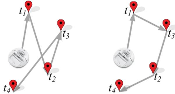
(a) The robot performs the tasks as soon as they are revealed. (b) The robot waits for four tasks and performs them as a bundle.
