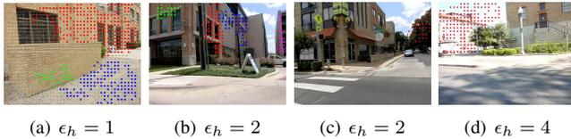
Fig. 6. Example of extracted planes. Dots with different colors indicate different extracted planes. (a-b) show all planes extracted in the frame. (c-d) show two incorrect extractions.
