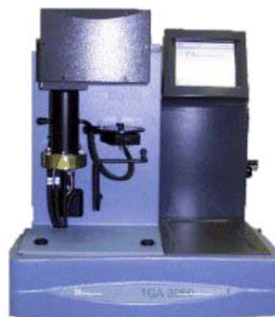
TGA Q500 with Autosampler
