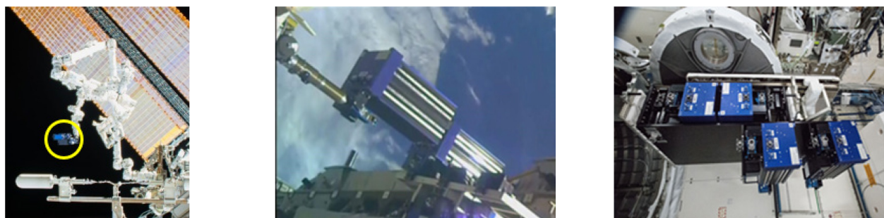
Figure 6: MISSE TT on the ISS robotics arm during transfer of SCs to the MISSE-FF (left, circled). Robotic SC installation on the MISSE-FF (middle). MISSE TT being brought back inside the ISS for crew to pack the SCs that have been installed/exposed on the MISSE-FF for return to Earth in a SpaceX Dragon.
