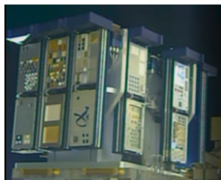
Figure 2: MISSE On Orbit. View of nadir face (right; one nadir SC slot is unoccupied) and ram face (left side of image). All SCs are opened.
