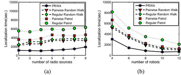
Fig. 4. Experiment results: (a) Localization time vs. number of radio sources. (b) Localization time vs. number of robots.
