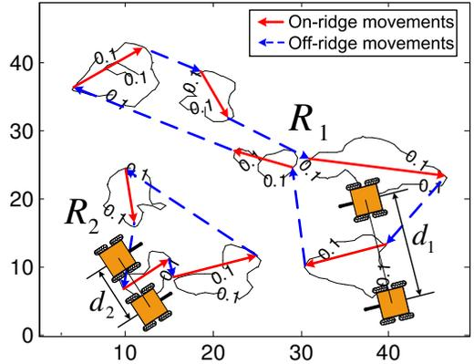
Fig. 3. An illustration of level sets with probability threshold of 0.1, ridges, and Pairwise Ridge Walking Algorithm with two pairs of robots over a  $50 \times 50$  grid.
